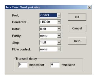
Figure 5-2 COM Port Configuration
