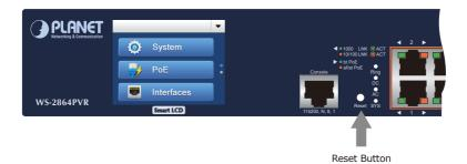
Figure 6-2 Reset button of WS-2864PVR
