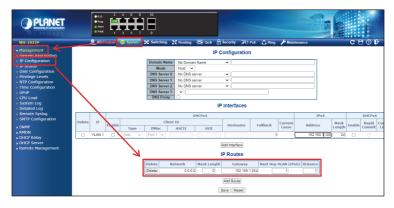
Figure 4-5 IP Configuration setting
