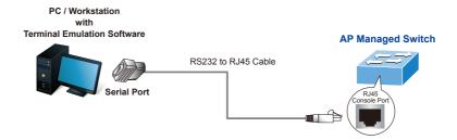
Figure 5-1 AP Controller Console Connectivity
