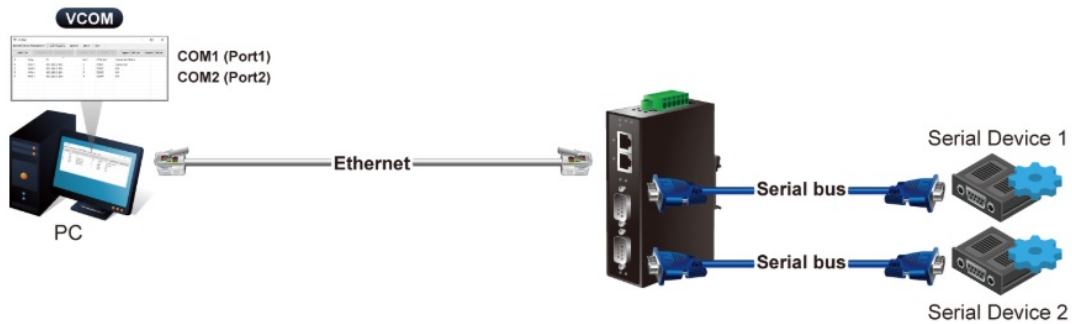
Figure 4-5-26: Virtual COM Mode Topology
