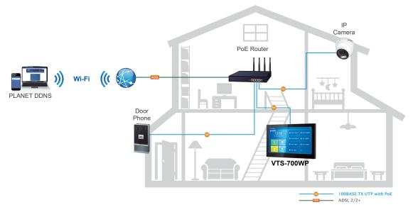
The system utilizes a 7" Touch Screen to get to the key functions with just one click to combine various household facility applications, including camera monitoring, access control, intercom, security, scene control, and value-added services, to bring you a new, comfortable and convenient lifestyle.
