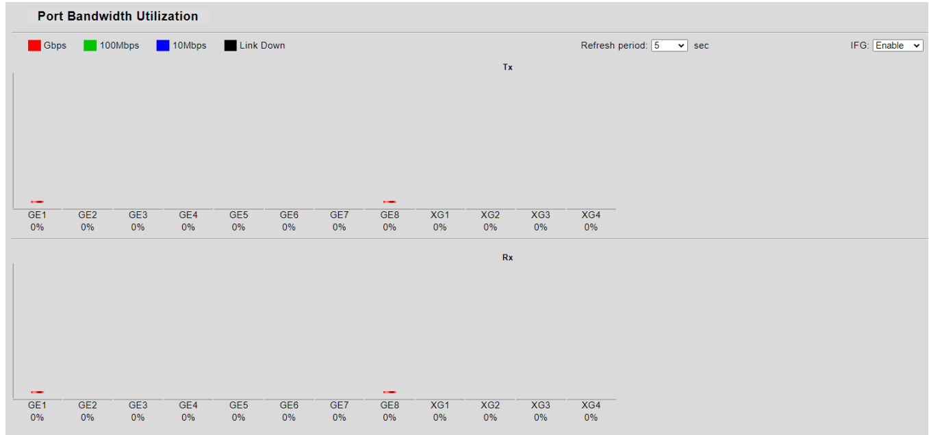
Figure 4-3-7: Port Bandwidth Utilization Page Screenshot
