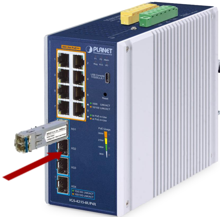
Figure 2-2-4: Plug in the SFP Transceiver
