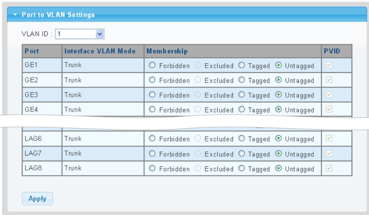
Figure 4-5-7: Port to VLAN Setting Page Screenshot
