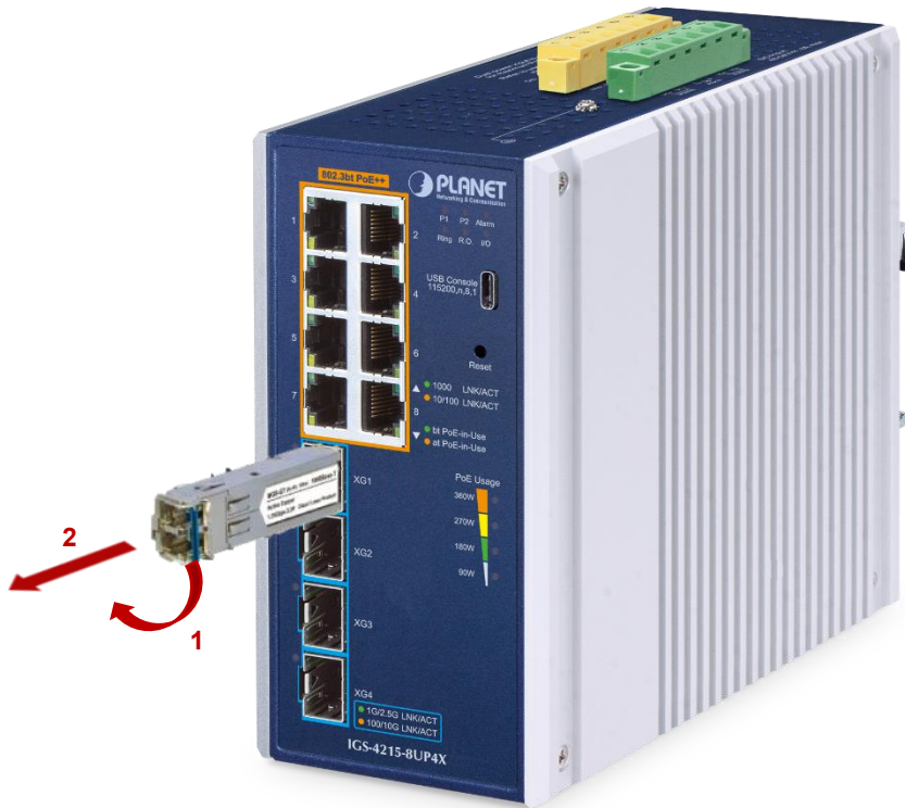
Figure 2-2-5: Pull out the SFP Transceiver Module
