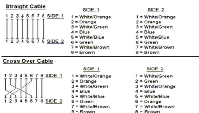
Figure A-1: Straight-Through and Crossover Cable
