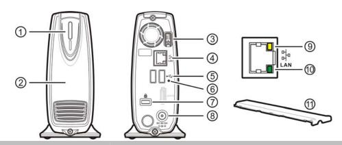
1 Power LED: Power and access (blue) / Booting-up or reset(orange)
