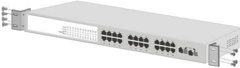
Figure 2-5 Attach brackets to the switch.
