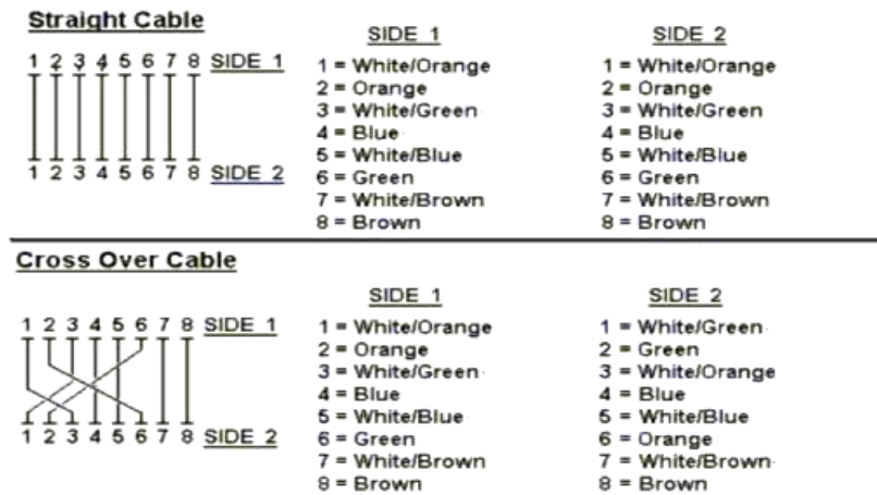
Figure A-1: Straight-Through and Crossover Cable
