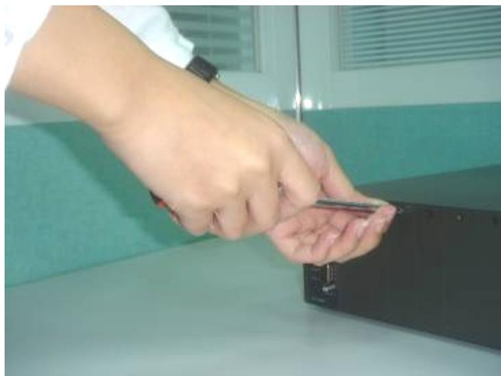
**Step 3:** Slide the FST-80x / GST-70x / GST-80x Media Converter board into the expansion slot, aligning it with the guide rails, until it firmly connects to the chassis' backplane.
