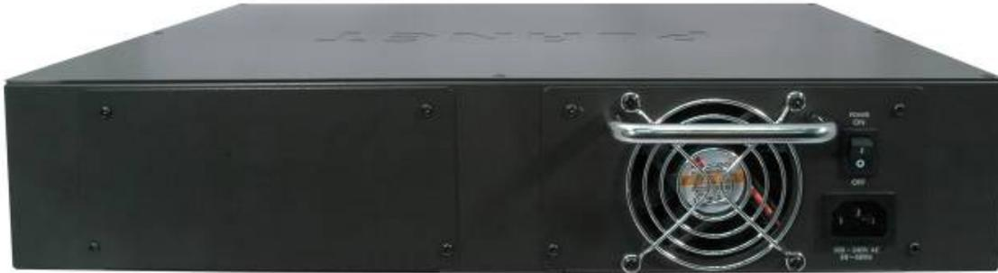
**Figure 2-3:** Rear panel of Managed Media Converter Chassis
