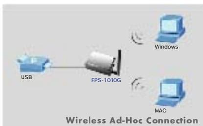
Work with the Wireless interface and configure the print server to "Ad-Hoc" mode. All wireless users can share the printer.
