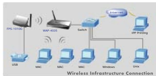
Work with Wireless interface and configure the Print Server to "Infrastructure" mode. All wired, wireless and Internet users can share the printer.
