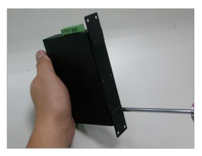
Figure 2-11 Attach brackets to the Industrial Equipment.
