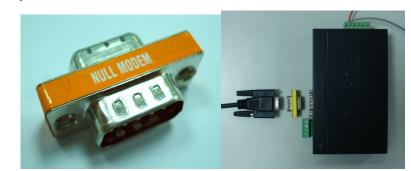
Once the Pair Connection mode of two ICS-210x be correctly configured but still fail link, check the RS-232 cables!
