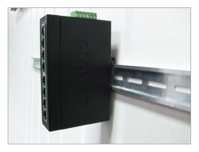
Figure 2-9 Industrial Equipment installed in DIN-Rail mount.
