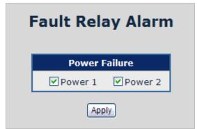
Figure 4-4 Fault Relay Alarm screen
