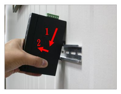
Figure 2-10 Remove Industrial Equipment in DIN-Rail mount.
