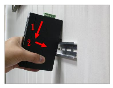
Figure 2-8 Install Industrial Equipment in DIN-Rail mount.
