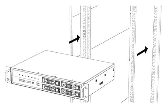
• Lock the server to the rack by mounting the ear brackets to the rack.
