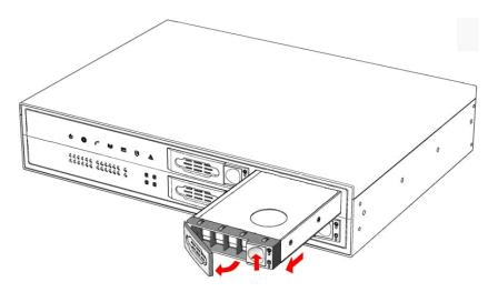
Mount the disk into the carrier and load the fixing screws.
