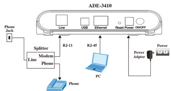
Figure 1: ADE-3410 connection diagram
