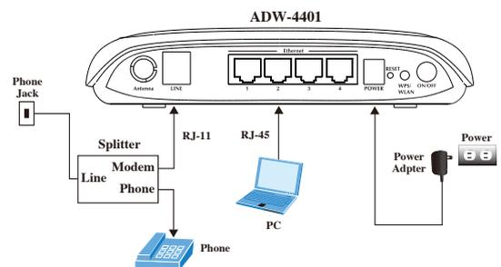
Figure 2: ADW-4401 connection diagram
