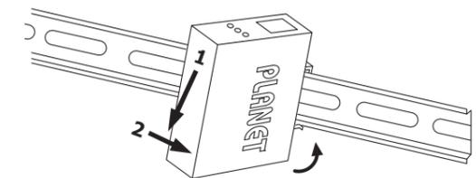
**Step 3:** Check the DIN-Rail is tightly on the track.
