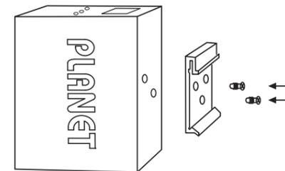
**Step 2:** Lightly press the button of DIN-Rail into the track.
