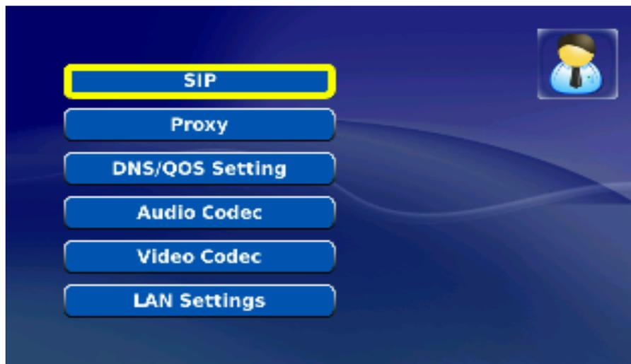
Need to input password (**1234**) and then you can enter to advance settings such as SIP, Proxy, DNS Setting, Audio Codec, Video Codec and LAN Settings.
