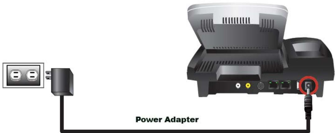
**Note: Only use the power adapter shipped with the unit to ensure correct functionality.**
