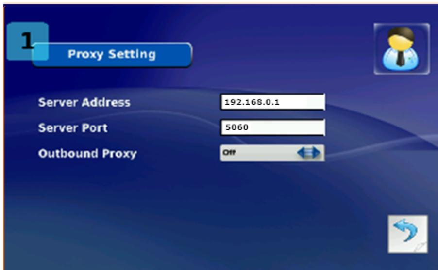
The screenshot shows the 'Proxy Setting' configuration page, indicated by a blue box with the number '1' in the top left. At the top left is a blue button labeled 'Proxy Setting'. In the top right corner is a user icon. The main area contains three settings: 'Server Address' is '192.168.0.1'; 'Server Port' is '5060'; and 'Outbound Proxy' is 'Off' with a dropdown arrow. A blue arrow icon is in the bottom right corner.
