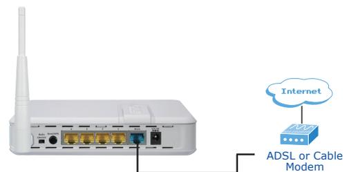
**STEP 3: Connect network devices to LAN port**
