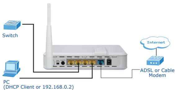
**STEP 4: Connect the Power. Check the LEDs on the front panel are on accordingly**
