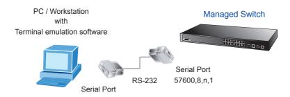
Figure 3-1 Serial / Console connection
