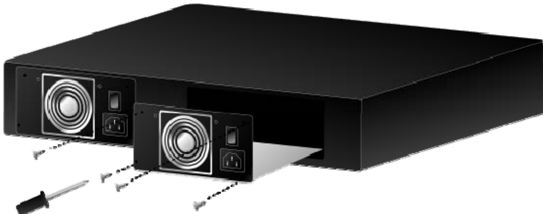
Figure 2-1-9: Install and remove the power supply unit of VC-2400MR series
