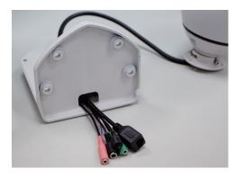
**Step 5:** Connect the camera and ring by locking the screws.
