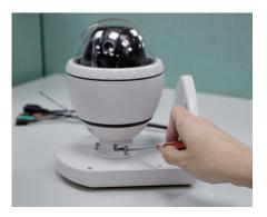
Step 8: Install whole stand with camera on the wall.
