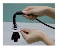
**Step 3:** Put the cable into the stand one by one.
