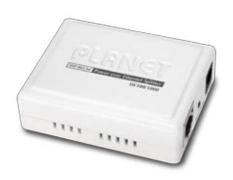
With cost saving and power management feature, PLANET POE-152S is a 10/100/1000Mbps Power over Ethernet splitter ideal for quick PoE environment deployment. The POE-152S can split the 48V DC over the Ethernet cable into 5V/12V DC power output. Working with the IEEE 802.3af power source equipment (PSE), the POE-152S frees the device deployment from restrictions of power outlet locations, which eliminates the costs for additional AC wiring and the installation time.
