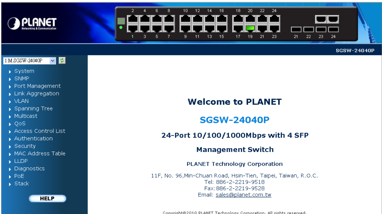
Figure 3-4 Web main screen of Managed Switch
