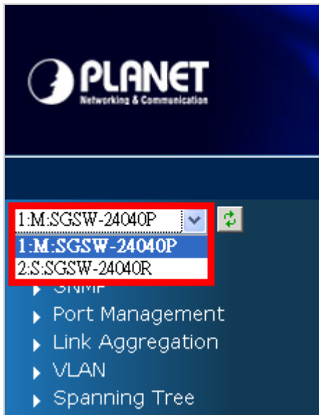
Figure 4-17-15 To manage the member switch
