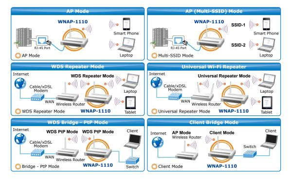
Being an access point, the WNAP-1110 supports the VLAN function to allow multiple SSID (Four sets of SSID) to access Internal VLAN topology. Moreover, its Wi-Fi Multimedia (WMM) capability provides enhanced QoS over wireless connection for better performance in multimedia transmission like on-line game and video streaming, which is classified as a top priority.
