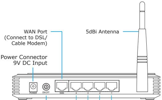
WAN Port (Connect to DSL/Cable Modem)
