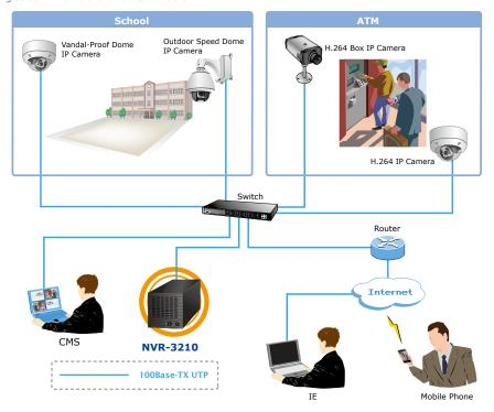
The NVR-3210 enables the administrators to simultaneously monitor the multisite surveillance up to 1024 channels\* via its bundled CMS software, multi-monitor and E-Map functions.
