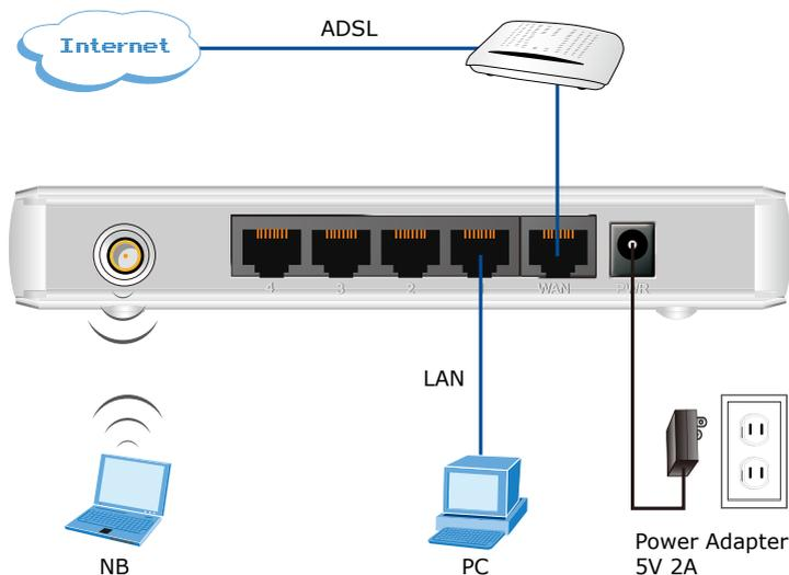
2) Then, you need to setup your LAN PC clients so that it can obtain an IP address automatically. By default the VRT-402N's DHCP server is enabled so that you can obtain an IP address automatically.
