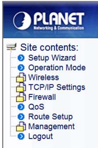
Figure 4-1 The Menu of Router Mode in The Web UI
