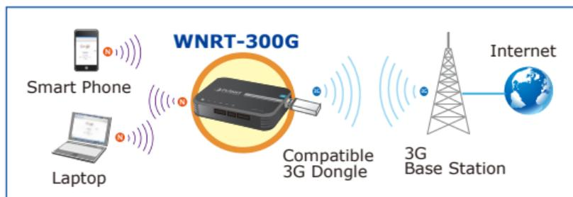
**Step 4:** Please use your PC to site survey the wireless signal of WNRT-300G, and connect your PC with it wirelessly.
