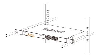
Figure 3-3: Mounting the PoE Fast Ethernet Switch in a Rack
