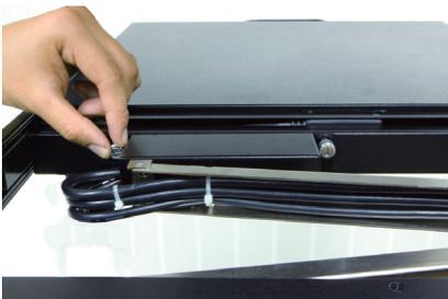
**STEP 6 : Pull and turn the lock knobs (left and right at the same time) then put out the screen and open console to operate**
