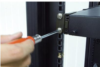
**STEP 3 : Screw the KVM module into the console from the back**
