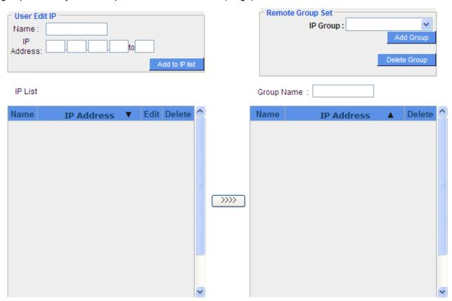
It is the same setting methods. You should set the IP address or the range of remote IP from the left side first, and choose to add IP address information from the left side into the remote group.
