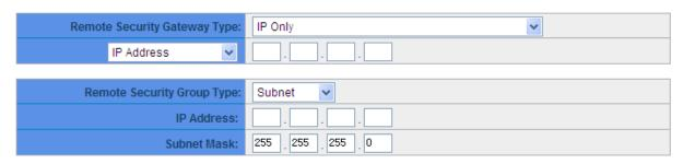
This remote gateway authentication type (Remote Security Gateway Type) must be identical to the remotely-connected local security gateway authentication type (Local Security Gateway Type).
