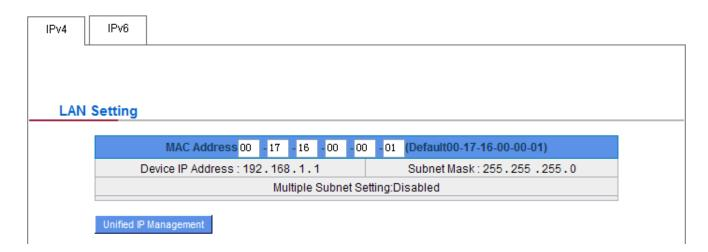
This is configuration information for SG-4800 current LAN IP address. The default configuration is 192.168.1.1 and the default Subnet Mask is 255.255.255.0. It can be changed according to the actual network structure.
