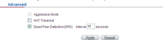
The advanced settings include Main Mode and Aggressive mode. For the Main mode, the default setting is set to VPN operation mode. The connection is the same to most of the VPN devices.
