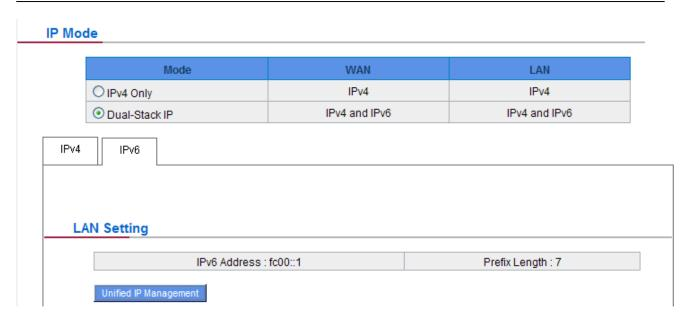
Click "Unified IP Management" to enter the configuration page, as shown in the following figure. Input the respective IP addresses and subnet masks.
