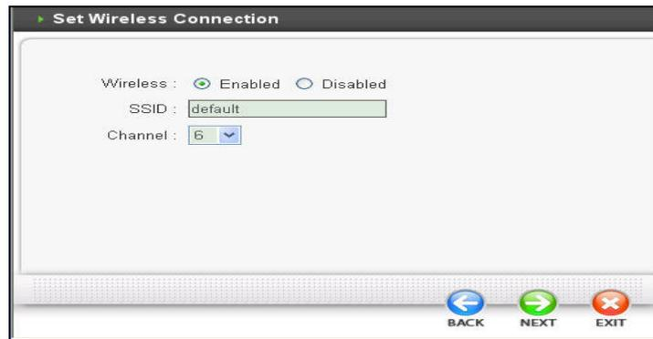
You can either enable or disable the wireless interface. If the Wireless LAN is enabled, you should set a ESSID and Channel for the wireless client to access . Click "NEXT" to continue.
