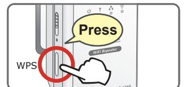
3. Wait for the connection being established. If connection is successfully established, the "WPS" LED will light for 5 minutes.
