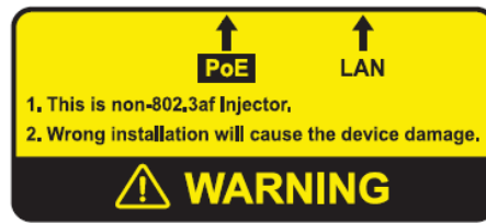
Figure 2-6 Warning Label of PoE Injector
