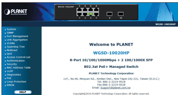
Figure 6-3: Web Main Screen of Managed Switch
