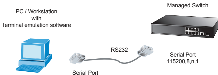
Figure 3-1: Managed Switch Console Connectivity
