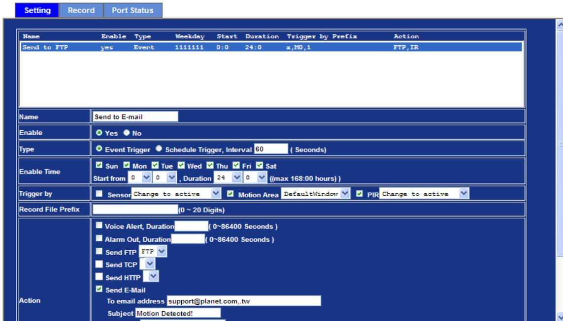
The screenshot shows the 'Setting' tab of the camera's web interface. At the top, there are three tabs: 'Setting', 'Record', and 'Port Status'. Below the tabs is a table with the following columns: Name, Enable, Type, Weekday, Start, Duration, Trigger by Prefix, and Action. The first row in the table is 'Send to FTP' with 'yes' for Enable, 'Event' for Type, '1111111' for Weekday, '0:0' for Start, '24:0' for Duration, 'x,MO,1' for Trigger by Prefix, and 'FTP,IR' for Action.
