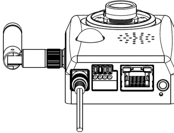
Once you have installed the IP Camera well and powered it on, the network accessing type LED will turn on. It means the system is booting up successfully. Furthermore, if you have a proper network connection, and access to the IP Camera, the LED will flash green under wired mode or orange under wireless mode.
