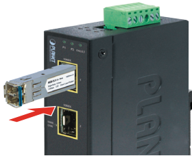
Figure 2-3: Plug in the SFP Transceiver
