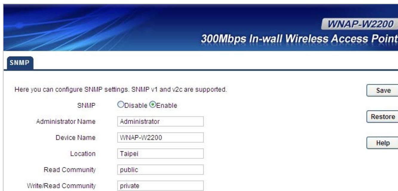
The screenshot shows the configuration page for the WNAP-W2200 300Mbps In-wall Wireless Access Point. The page title is "WNAP-W2200 300Mbps In-wall Wireless Access Point". The "SNMP" tab is selected. The page contains the following configuration options:
