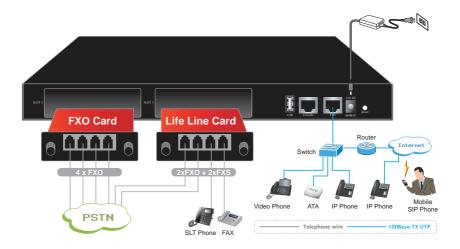
Figure 2-3 Physical Connection Topology of the IPX-2100
