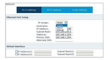
Figure 3-4 Selection of IP Connection Type
