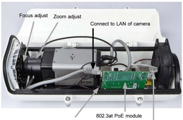
Provide power to camera, heater, IR LED and blower
