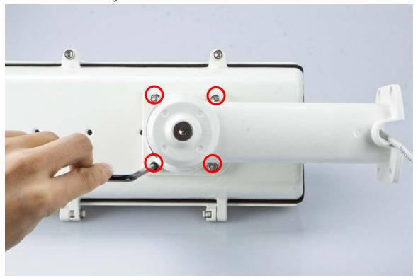
**2.2.5** After the above steps have been done, place the ICA-2250VT on the wall with the four screws tightened.
