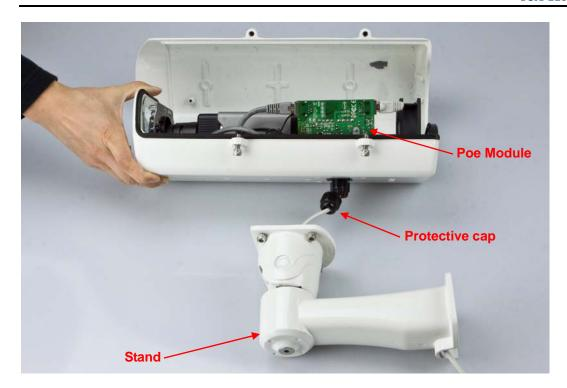
**2.2.3** Use the wrench from the wall mounting kit to clockwise tighten the screw and protective cap.
