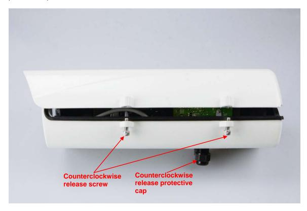
**2.2.2** Slide an RJ-45 cable without its plug through the stand and the protective cap. Then fix the RJ-45 plug and connect it to the connector of the PoE module. Please note that the whole RJ-45 cable (with the plug) cannot go through the protective cap. When the setup is completed, user can use PoE tester to test PoE module to check whether the LED works or not.
