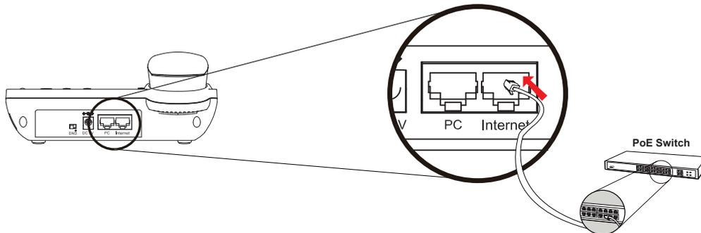
**NOTE :** Only internet port of the VIP-256PT support 802.3af power injection, use of any non-standard POE injector could damage the device.
