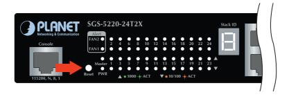
Figure 8-1: Stackable Managed Switch Reset Button
