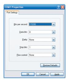
Figure 3-2 COM Port Configuration
