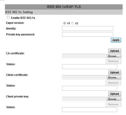
IEEE 802.1x is an IEEE standard for port-based Network Access Control. It provides an authentication mechanism to device wishing to attach to a LAN or WLAN.
