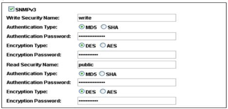
For data security reason, the authentication and encryption assurances are added when developing SNMPv3. The user has to give not only the security name (the same as
