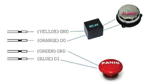
A. Please connect the G & DO pin to the external relay (buzzer) device When no event happens, DO output is 5V (DO and GND are disconnected). When the camera detects event happening and triggers external alarm, DO output is 0V (DO and GND are connected).
