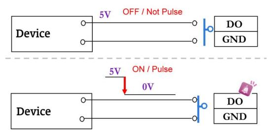
B. Please connect the G & DI pin to the external trigger device.
