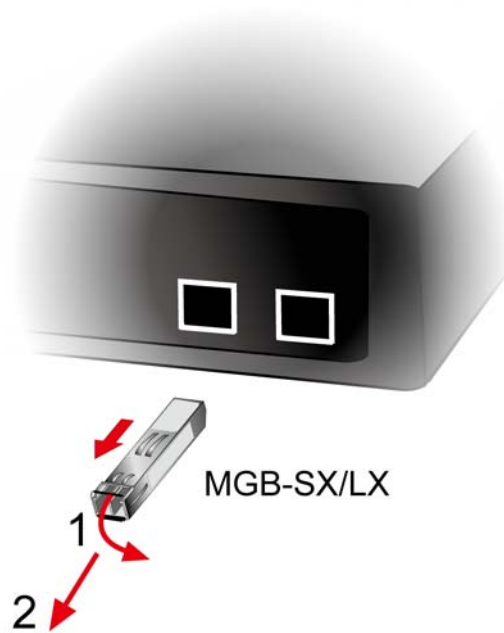
Figure 2-1-8 How to Pull Out the SFP Transceiver
