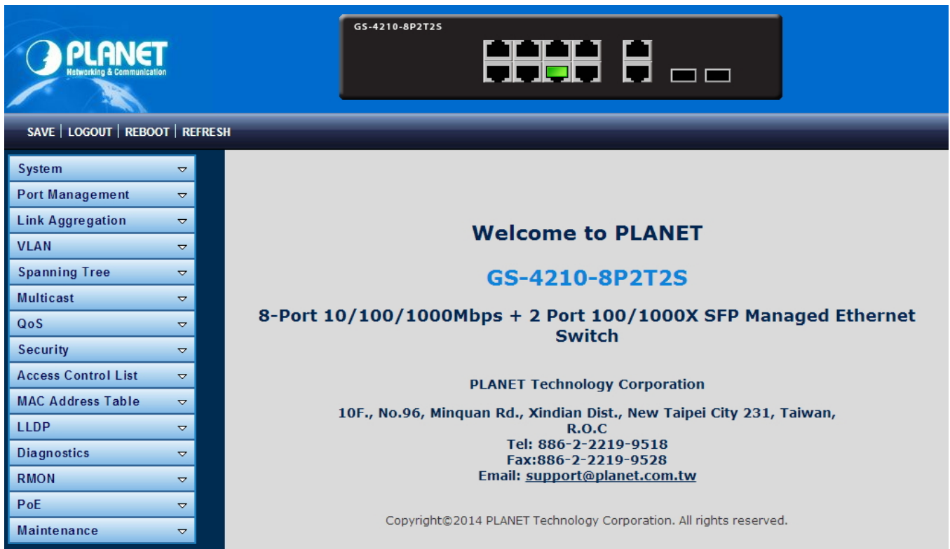
Figure 3-1-4 Web Main Screen of Managed Switch
