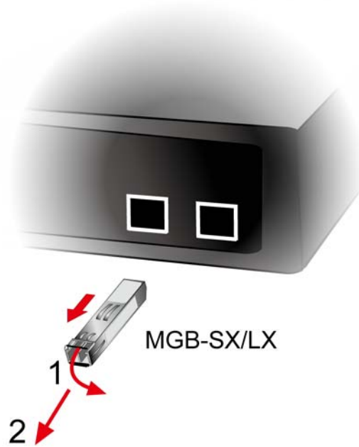
Figure 2-2-5: How to Pull Out the SFP/SFP+ Transceiver
