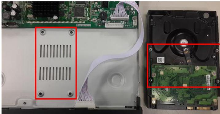
**Step 4:** After the HDD is secured, it should look like the one in the pictures (front and back) below:
