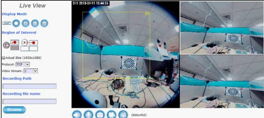
Scrolling the mouse wheel could change region's magnifying power (x1 to x10); and dragging the frame with mouse could move the amplified region. At the same time, you can also see region's amplification effect displayed real time in the lower-left, upper-right or lower-right Live View Window.
