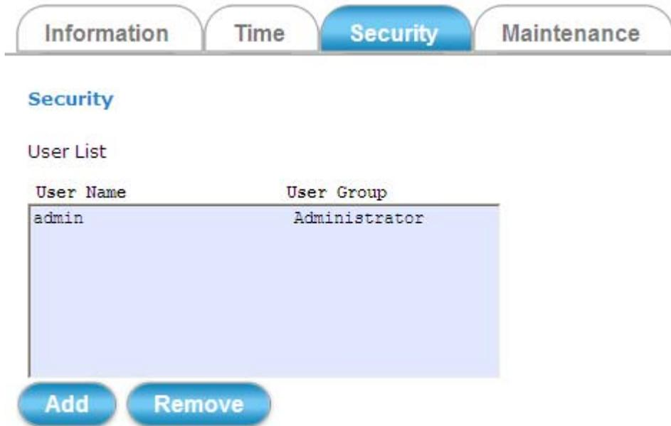
The **Security** tabbed pane allows you to add new camera User Name and change Password and the surveillance status or User Group. Click the **ADD** button to access the security setup dialog (shown below).
