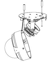
4. To adjust lens, move the camera body by pan and/or tilt manually and set the zoom/focus by turning the lens to the left or right direction.
