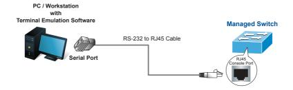
Figure 3-1: Managed Switch Console Connectivity
