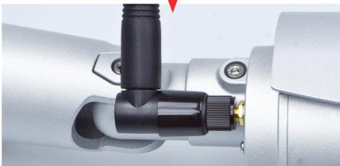
b. Push the **Rubber Cover** until it could totally cover the antenna connector. It is helpful to prevent water.
