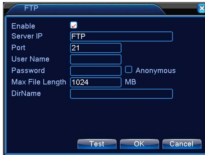
Picture 5.23 FTP Setup
