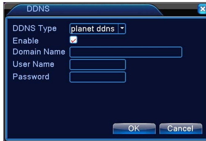
Picture 5.22 DDNS Setup
